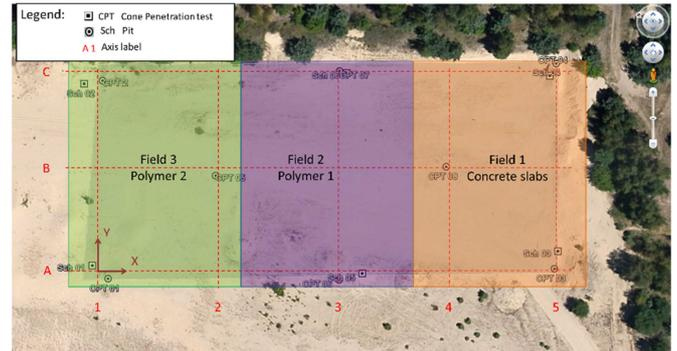
Fig. 5 Test area with sub-fields and main investigation points [5]
