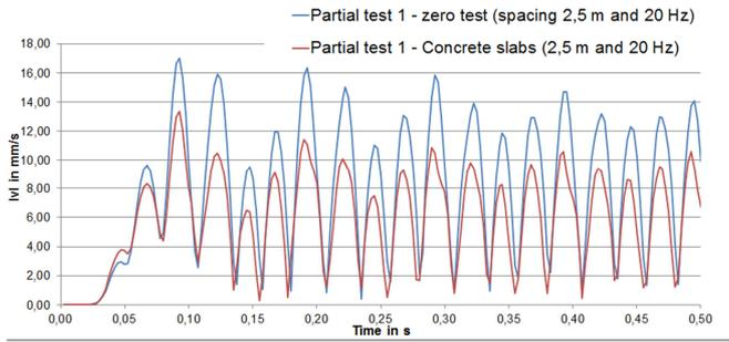
Fig. 9a Exemplary results – Partial test 1
