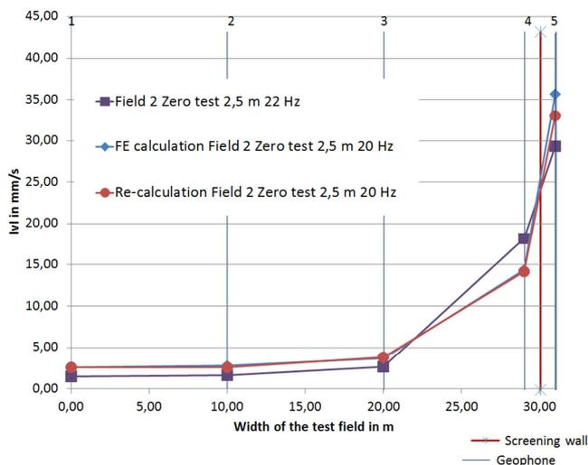
Fig. 11b Exemplary result of the recalculation – Field 2
