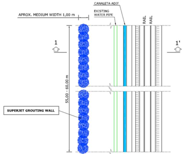
Fig. 3a Plan view – Soilcrete® as a vertical wave barrier
