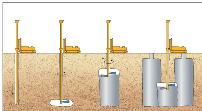
Fig. 1a Soilcrete® (drilling, cutting, soilcreting, extending)
