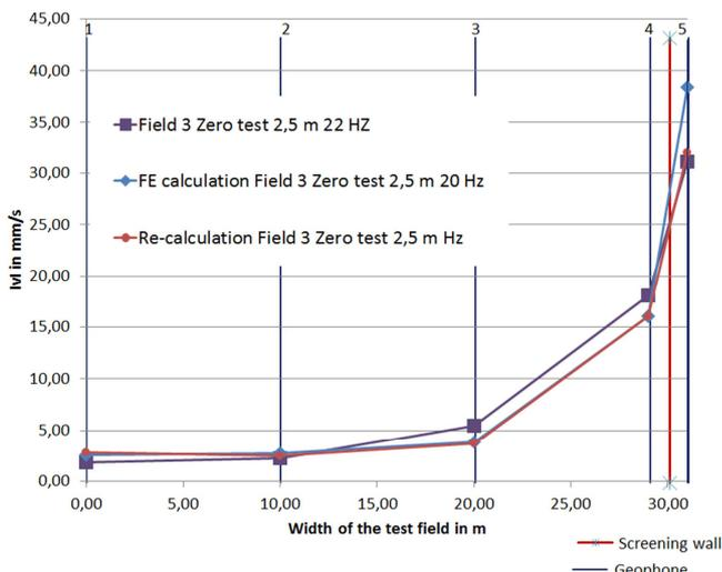
Fig. 11c Exemplary result of the recalculation – Field 3
