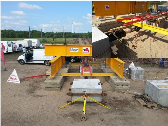
Figure 1. Computer controlled hydraulic jack for rapid horizontal loading in two directions.(upper right) and overview of test setup for dynamic horizontal excitation of one pile group under constant vertical load.
