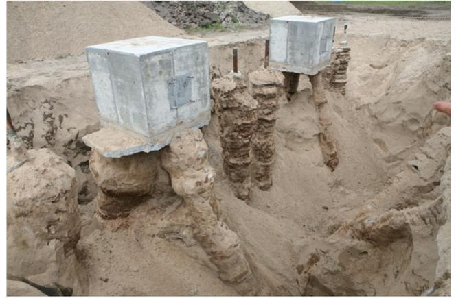
Figure 8. Excavated test foundations after the field tests.
