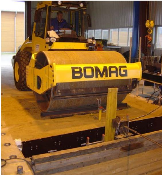
Figure 9: Large scale experiment "Cottbus", Dynamic loading
